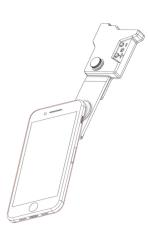
Place the lens tile on the subject to observe. **Keep DIPLE Lux in one** hand, like a magnifying lens, and the phone on the other hand. With the camera-app on, move the phone toward the centre of the black rubber ring and get in contact with it. Slightly tilt the DIPLE Lux, or use the elevation screw in the tile to find the right working distance. Change the light intensity with the buttons + and -.
