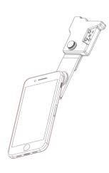
Place the lens tile on the subject to observe. **Keep DIPLE Lux in one** hand, like a magnifying lens, and the phone on the other hand. With the camera-app on, move the phone toward the centre of the black rubber ring and get in contact with it. Slightly tilt the DIPLE Lux. or use the elevation screw in the tile to find the right working distance. Change the light intensity with the buttons + and -.
