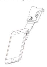
Place the lens tile on the subject to observe. Keep DIPLE Lux in one hand, like a magnifying lens, and the phone on the other hand. With the camera-app on, move the phone toward the centre of the black rubber ring and get in contact with it. Slightly tilt the DIPLE Lux, or use the elevation screw in the tile to find the right working distance. Change the light intensity with the buttons + and -.
