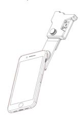
Place the lens tile on the subject to observe. Keep DIPLE Lux in one hand, like a magnifying lens, and the phone on the other hand. With the camera-app on, move the phone toward the centre of the black rubber ring and get in contact with it. Slightly tilt the DIPLE Lux, or use the elevation screw in the tile to find the right working distance. Change the light intensity with the buttons + and -.
